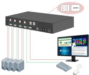
The Roaming-Mouse feature provides the user simply moves the mouse cursor across screen borders in any direction, either horizontally or vertically, instantly selecting the PC they need to control – providing super easy-to-use KVM switching that saves time and desk space.
