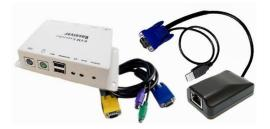
The Kit effectively extends PC KVM (Keyboard, Video and Mouse) control to the Console Receiver and also provides for convenient single access; in addition to the remote console access, you can also connect a monitor/ keyboard/ mouse set to provide local PC access.
